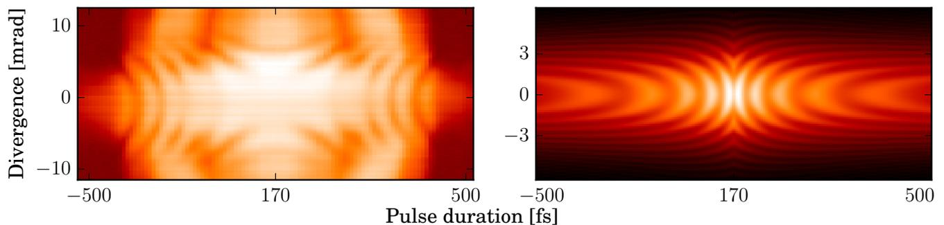
**Figure 1:** *Spatial lineouts of the 17th harmonic of 1030 nm, for different pulse durations. A negative sign of the duration corresponds to negative chirp (red edge first, blue edge last) and vice versa. To the left, experimental data are shown, while to the right, the results from the simple Gaussian model are shown.*
