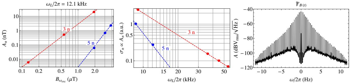
**Figure 1:** Left and central graphs show the  $A_n \propto B_{\omega_{exc}}^n$  and  $\sigma_n \propto \omega_L^{-(n-1)}$  dependencies of the multiphoton process, respectively. The right graph shows the Fourier spectrum of a 157 Hz square-wave modulated  $B(t)$  field measured by a self-oscillating magnetometer.
