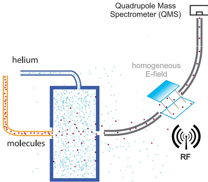
Figure 1: *RF spectroscopy setup*
