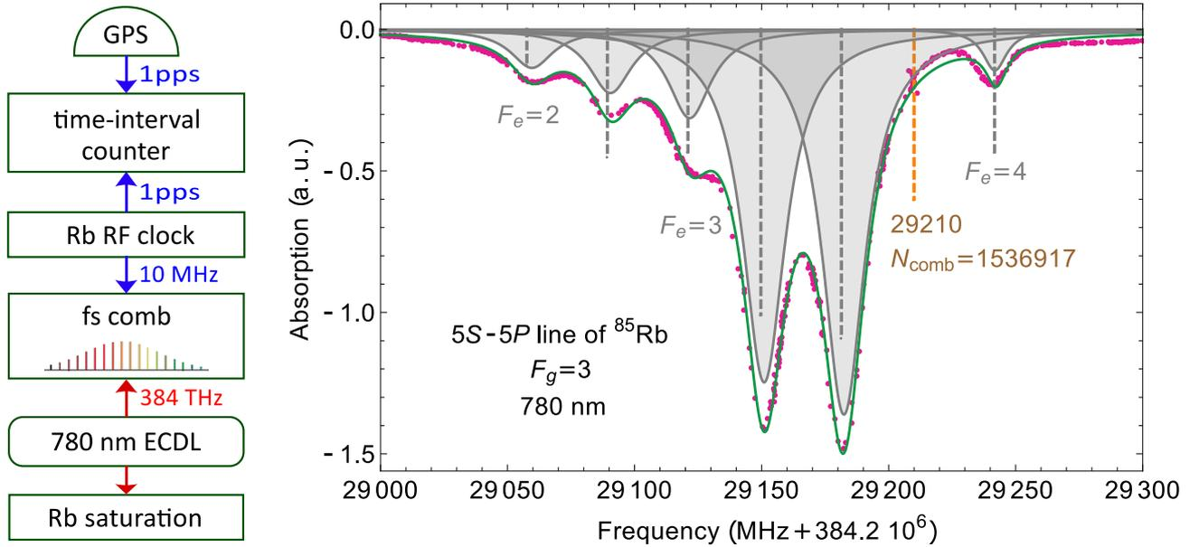
**Figure 1:** *Left: Experimental scheme. Right: Precision measurement of absolute frequencies of Rb saturation peaks using optical frequency comb. Multiple peaks fitting using Lorentz functions is shown.*
