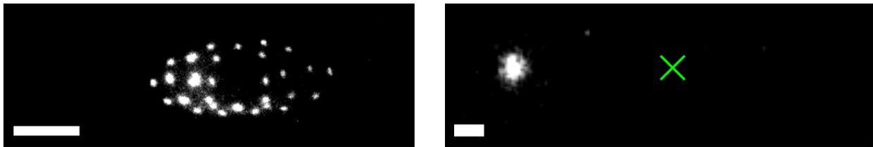
**Figure 1:** *Left: A single  $\text{Ar}^{13+}$  ion sympathetically cooled by several  $\text{Be}^+$  ions. White scale bar denotes 100  $\mu\text{m}$ . Right: A single  $\text{Ar}^{13+}$  ion (position marked by cross) sympathetically cooled by a single laser-cooled  $\text{Be}^+$  ion. White scale bar denotes 20  $\mu\text{m}$ .*
