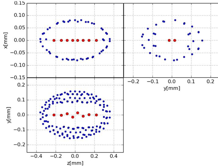
**Figure 1:** Sympathetically cooled  $Ar^{13+}$  (5 ions) by laser cooled  $Be^+$  (256 ions). The HCI are in a zig-zag structure while the Be ions form a 3D crystal around.
