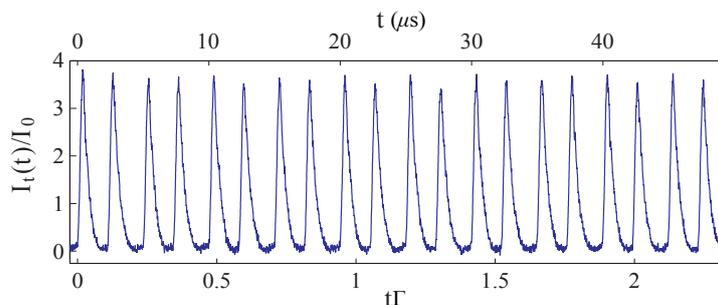
**Figure 1:** An example of a pulse train generated in our experiment. The repetition time of this pulse train is  $0.12\Gamma^{-1}$ , which is shorter than the lifetime of the transition, showing that cooperative effects are at play.
